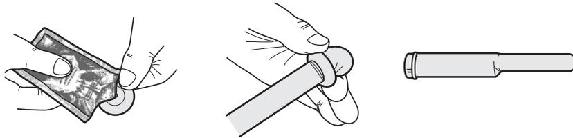
2. Mount the biopsy adapter onto the probe. If the surface of probe is fluted, mount the adapter in accordance with it.
