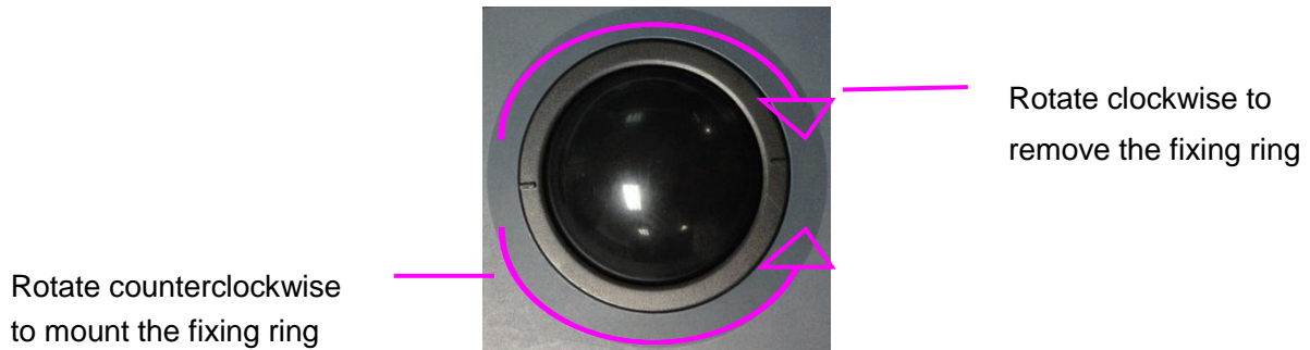
Figure 13-1 Assembling and Disassembling Trackball
